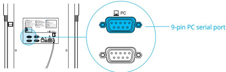
If there is no serial port on your PC, you can connect a normal USB-AB type cable to the USB SLAVE port on the rear of InBody770 instead, and connect the other end of the USB cable to the USB port of the PC.
