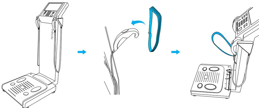
5. Slightly lower the upper part of the InBody770 and hook the Packing Band to the leveling screws as illustrated below.
