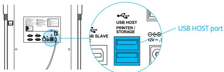
3) Turn on the InBody770. If the barcode reader is connected to the InBody770, the barcode reader icon (
