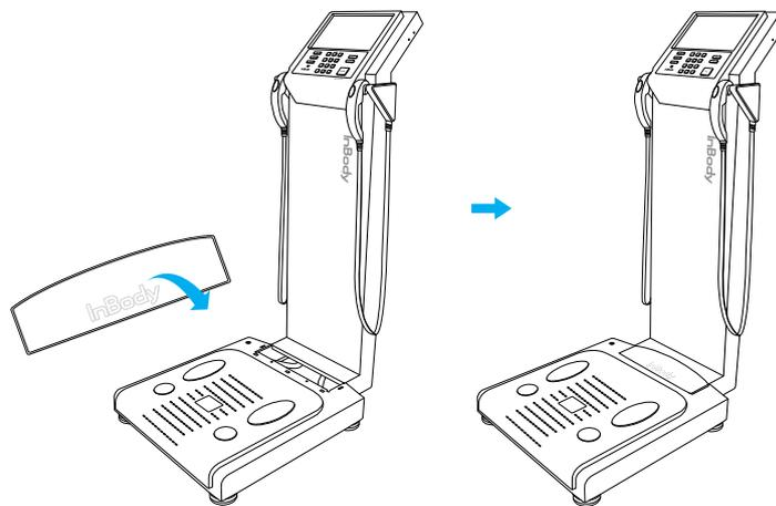
8. Level the InBody770 by rotating the leveling screws under the footplate to the left and right so that the air bubble is centered.
